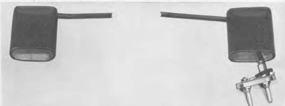
FIGURE 1. Photograph of the shielded plug and cable. TYPE 274-NE Shielded Plug and Cable consists of the two shielded terminals, as shown, connected by three feet of shielded cable. TYPE 274-ND Shielded Plug Assembly is one double terminal plug with shield. In the photograph the method of construction is shown by the disassembled terminal at the right.
