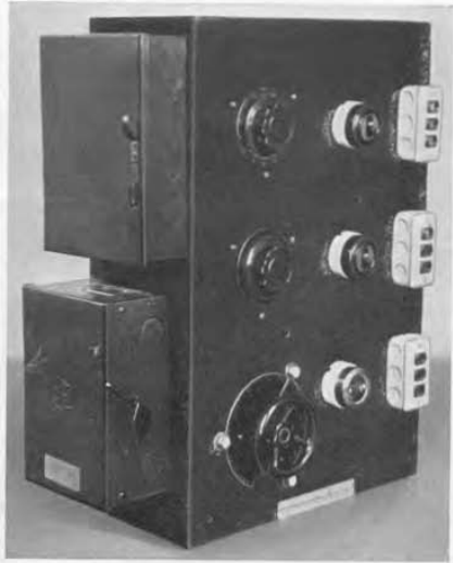
FIGURE 3. This experimental board uses one TYPE 100-K and two TYPE 200-CU Variacs. The total cost of parts for this assembly, in addition to the Variacs, was only $5.
